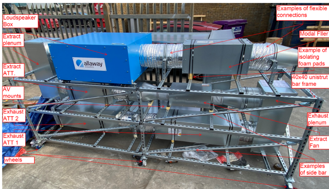
Figure 2 Test rig at the factory before it was cladded with acoustic insulation
