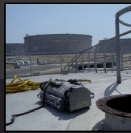
The RobTank robot on the roof of an oil tank in Portugal
