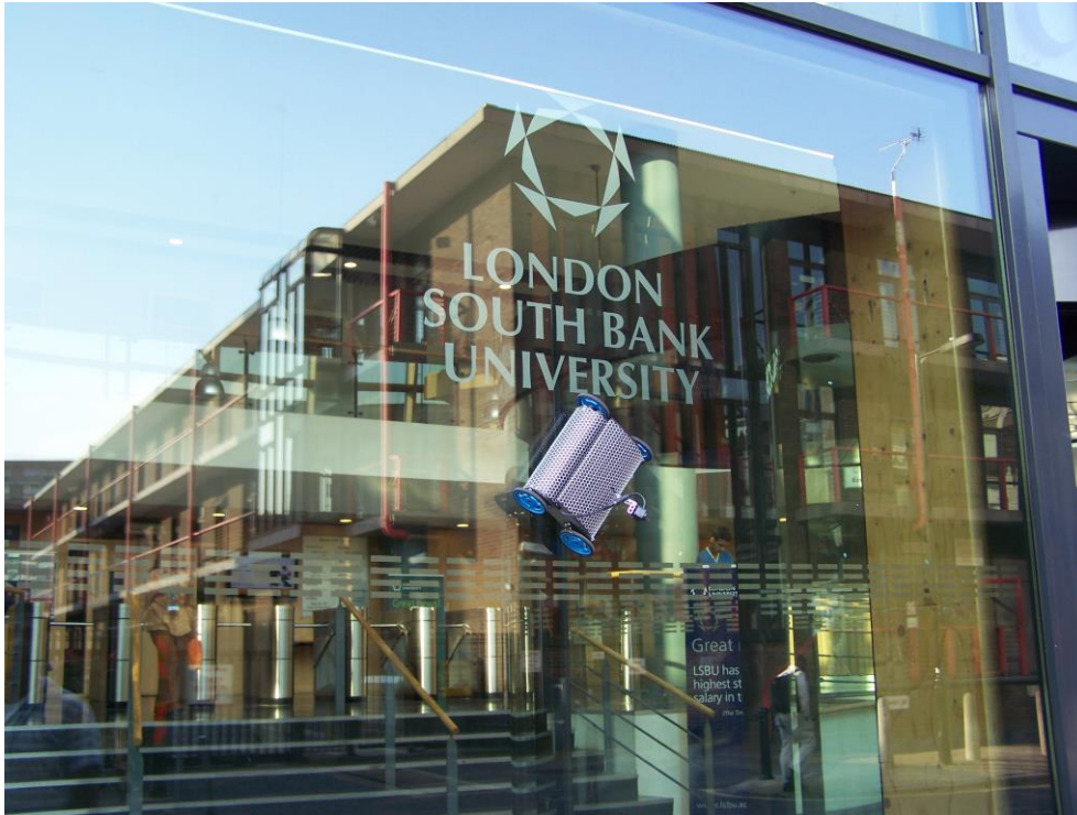
Figure 6: The Vortex robot with a vision system climbing on the glass front of the Keyworth building
