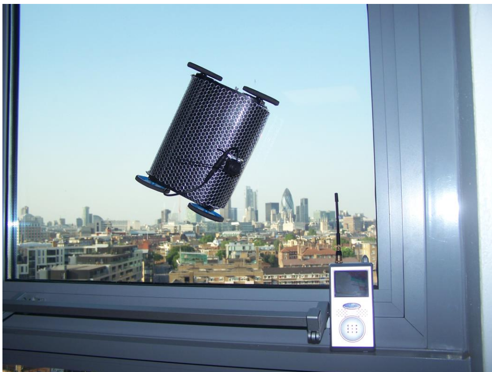
Figure 3: Vortex robot climbing on glass with vision system sending images to hand-held controller
