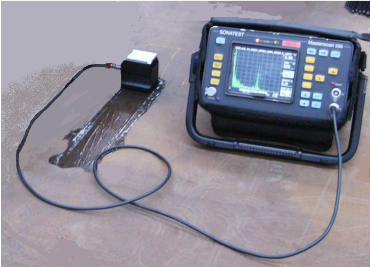
Figure 13: Ultrasonic testing hands-on display to find a hidden hole defect in a test block.
