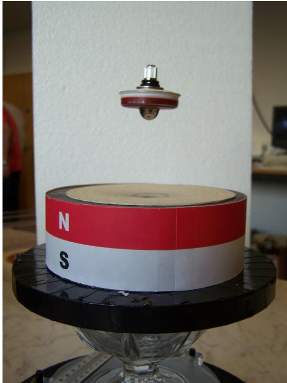
Figure 12: Spinning disc magnet levitating above another ring magnet
