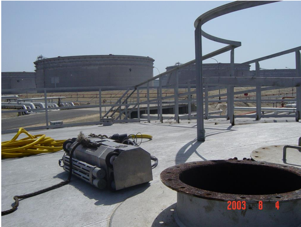
Figure 8: The ROBTANK storage tank floor inspection robot
