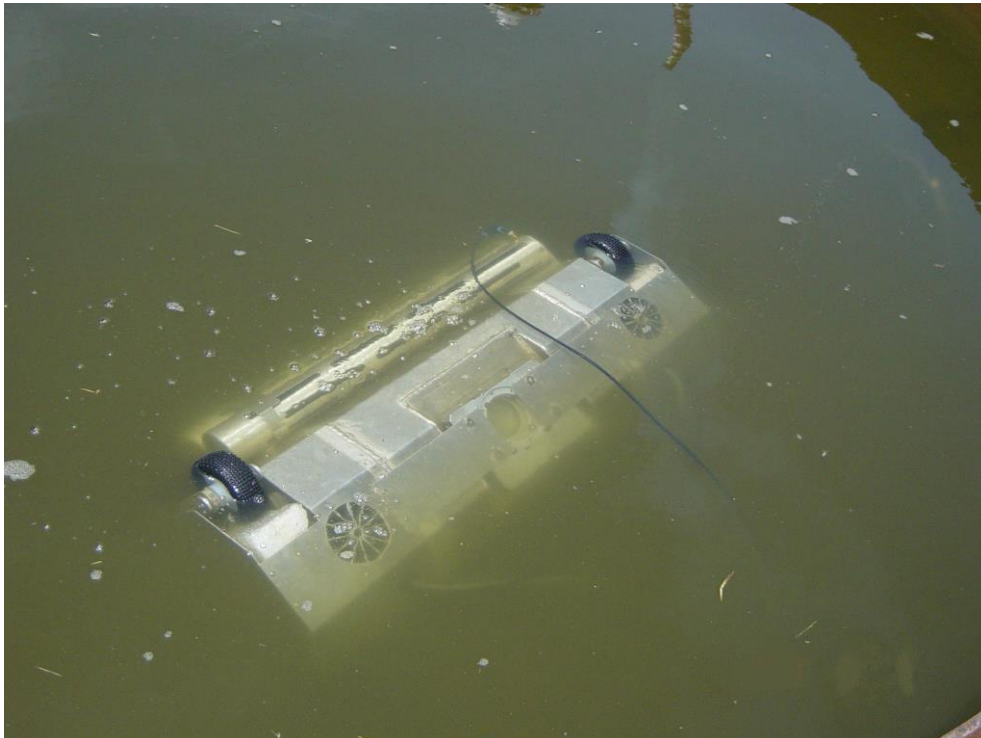
Figure 9: ROBTANK immersed in water in a fire fighting tank in the Sines refinery.
