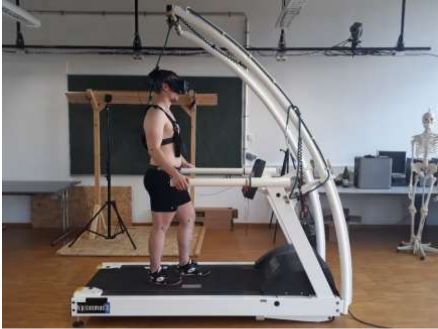
Fig. 2. Measurement setup on the treadmill with a participant wearing markers. The participant is safeguarded against fall by a safety belt on the upper body attached to the beam of the treadmill.
