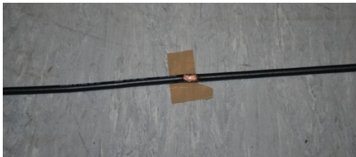
Figure 3. Fault created at around two meters from end of the six meter long cable (the position shown in Figure 2).
