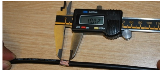
Figure 4. Shape and size of the 10 mm fault created on the insulation and braiding of an RG59 coaxial cable.
