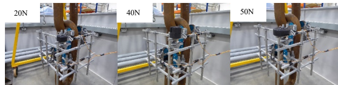
Figure 10. Stability test with external loads
