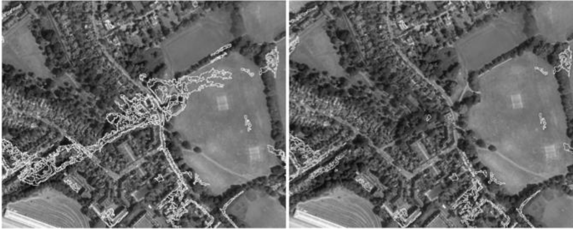
Figure 2. Flooded areas with (right) and without (left) the influence of SuDS. Base map taken from Google Earth.
