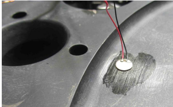
Figure 10 Sensor position on dish of planet carrier
