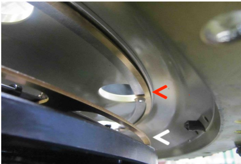
Figure 12 Coils in position before re-joining top cover (static coil red arrow, moving coil white arrow)
