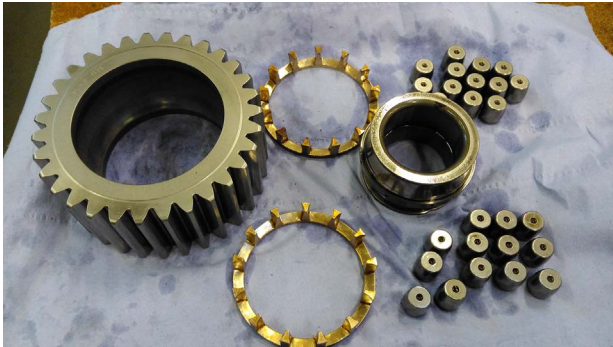
Fig. 6. The components of 2nd planetary bearing.
