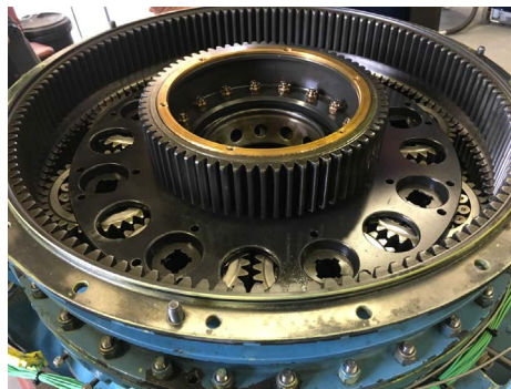
(b) 2 nd Epicyclic module ring and sun gears
