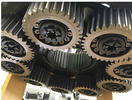
(a) 2 nd Planetary gears/ bearings
