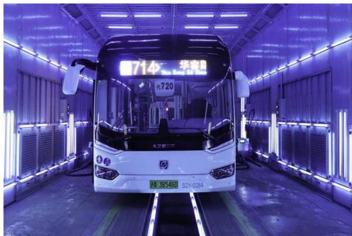
Figure 8: A passenger bus being disinfected by UVC in Shanghai, China. Reprinted with permission from [38]
