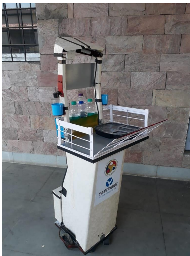
Figure 20: A prototype demonstrator of COPARBOT (Courtesy: Dr. S. Kanagaraj at IIT Guwahati, India)
