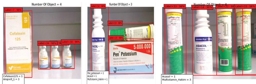
FIGURE 13: The output of the software is to identify and count the items in the image.
