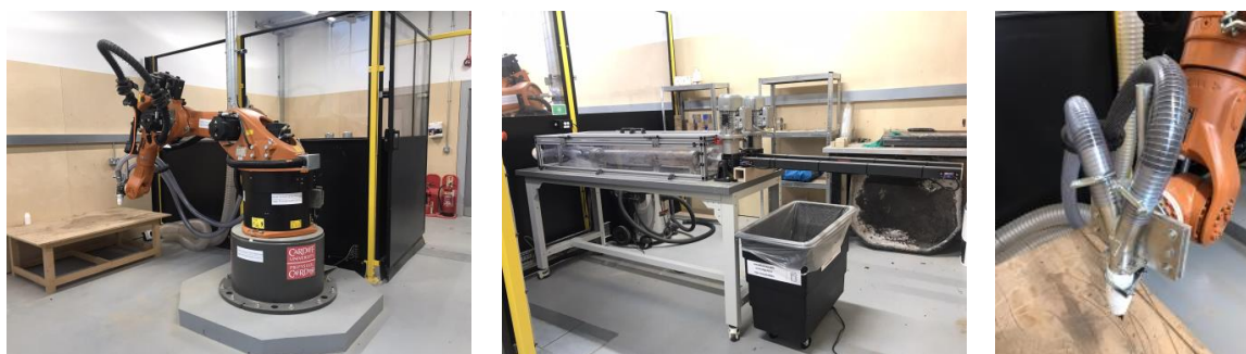
Figure 11,12,13. KUKA KR60 six axis high accuracy industrial robot, the dual extruder [16] and the custom fabricated steel end effector connecting 3D printed nozzle to the pressure hoses.
