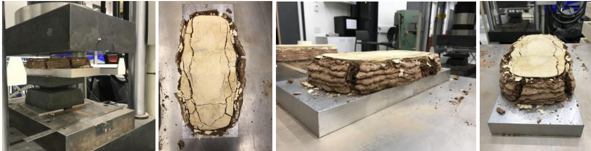
Figure 21. Typical failure at the corners and along the perimeter was observed for all specimens
