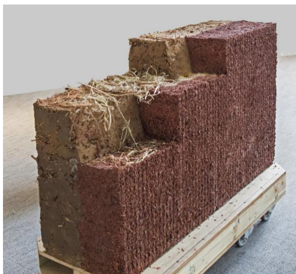
Figure 4: CobBauge wall sample (Goodhew et al [23]) Image courtesy of Llyod Russell and Steve Goodhew, University of Plymouth, all rights reserved.
