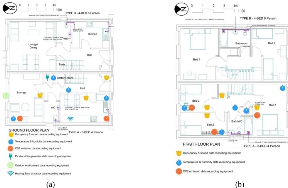
Fig. 3. (a) The tested and simulated ground-floor areas; the locations of the installed recording equipment for indoor and outdoor environmental conditions are indicated. (b) The tested and simulated first-floor areas.
